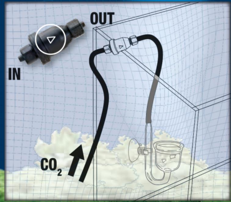
**FR CLAPET ANTI-RETOUR POUR LES INSTALLATIONS DE CO<sub>2</sub>**
